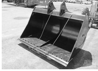
Fleco 330D bkt., ditch cleaning, 84" bkt., 3.25-yds., 100mm pin holes w/16-1/2 between ears & 23" center to center, bolt on cutting edge. .... $6,950
