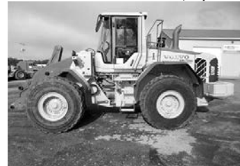
'10 Volvo L110F whl. ldr., rblt. eng., 4-yd. GP bucket, quick coupler, aux. hyd., ride control, 4 spd. powershift, tight center, orig. paint . . . . . $69,500
