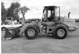
'12 Case 621F , cab, heat, A/C, bias ply 20.5x25 tires, tight center, 4 spd. pwr. shift, Cum. pwr., pin on 3-yr. bkt., nice, clean machine, 13,500 hrs. .... $49,500
