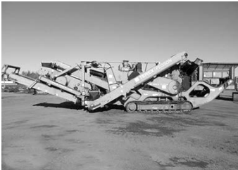
'07 Terex Pegson 4242SR, 428 fixed mill impact crusher, wear plates @ 50%, 1067mm x 711 mm vibrating feeder, side discharge, closed circuit, 5x12 screener. . . . . $169,500
