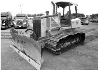
'13 Deere 700K LGP, OROPS, new U/C, pads @ 60%, strong running machine, tight 6-way blade, cutting edge 50%, Hystat variable spd. trans., clean . . . . . $69,500
