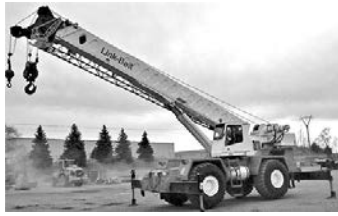
Link Belt 50-ton rough terrain crane , Cum. 6CT8.3-C, 35'6", 110' 4-sec. boom, 34'-56' swg. away extendable jib, Johnson 50-ton 3-sheave 1003 lb. block, 8.5 ton 378 lb. ball . . . $89,500
