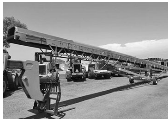
'06 Kimco 30x80 stainless conveyor , S/A, pintle hitch, hyd. cyl. raise & lower, hyd. driven conveyor, no hyd. pwr. .... $27,500
