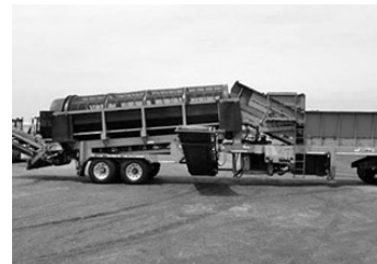
Wildcat RHC6230 trommel , 2-product screener, rear spoils conveyor, side discharge product conveyor, new belly conveyor, rblt. feed chain .... $59,500
