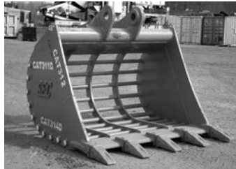
Sec 48" skeleton bucket 311, 312, 314, 65 mm pin holes w/8.7" between ears, 16" center-to-center . . . . $3,400
