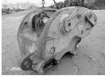
Cat CB 324, 325, 328, 329 hyd. quick coupler, 1134 lbs., 90mm pin holes w/13-7/8 between ears & 19-1/2 center to center. .... $3,950
