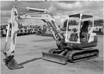
'08 Takeuchi TB250, 10,000# machine, frt. blade, swivel boom, 40 hp, good tracks, 2 spd. tracks, aux. hyd., quick attach, work ready machine . . . $27,500
