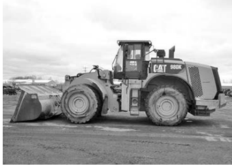
'14 Cat 980K whl. ldr., forestry pkg., extra rear wts., 3rd function hyd., 29.5R29 tires, tight center, frt. linkage tight, no frt. attachment, log grapple removed, 4 spd. powershift trans. . . . . $199,500
