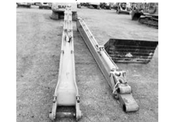
ELK 320 long reach boom , long reach for Cat 320 34' boom & 24' stick, 60" ditching bucket, fits Cat 320, 320B, 320BL, 320C, 320CL & 320D . . $19,500
