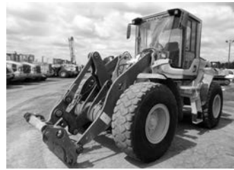
'09 Volvo L60F whl. ldr., 2.5-yd. bucket, quick coupler, 4 spd. powershift, tight center, has some minor bucket play, orig. paint . . . Quick Sale $45,000
