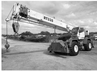
'98 Terex RT335 rough terrain crane, 4x4, (4) whl. steer, 6 spd. powershift trans., Cum., 35-ton, 30'-94" boom, 30' jib boom, (2) block sheave, aux. winch line, 23.5x25 tires @ 60%, 9500 hrs. . . . . $59,500
