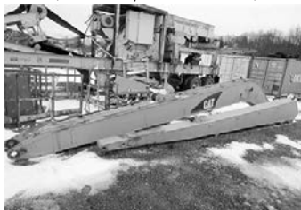
Cat 320 long reach 50' booms, boom & stick, 29' long boom, stick is 20'7" long, boom to house pin 90mm w/27" base width. . . . . $12,500
