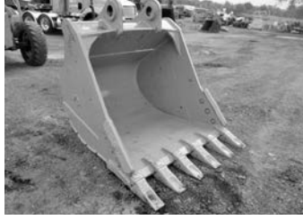
EMAQ 60" Cat 345 GP bucket, for Cat 345 TB linkage, 110mm pin hole & 100mm pin hole w/17-1/4 between ears & 23-1/2 center to center. .... $6,950
