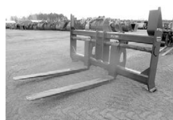
Doosan fork , 106x72 long forks, 7" wide by 3" thick, 39" center to center on hooks, 2880 lbs. .... $5,100
