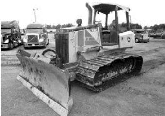
'13 Deere 700K LGP, EROPS, new U/C, pads @ 60%, strong running machine, tight 6-way blade, cutting edge 50%, Hystat variable spd. trans., clean ..... $69,500
