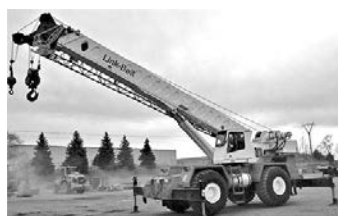
Link Belt 50-ton rough terrain crane, Cum. 6CT8.3-C, 35'6", 110' 4-sec. boom, 34'-56' swg. away extendable jib, Johnson 50-ton 3-sheave 1003 lb. block, 8.5 ton 378 lb. ball . . . $84,500
