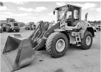
'13 Volvo L60G, EROPS, heat & A/C, quick coupler 3-yd. bucket, ride control, kick out options, float control, 20.5R25 rubber @ 60%, back up camera, strong runner, straight, clean, orig. paint. . . . . $69,500
