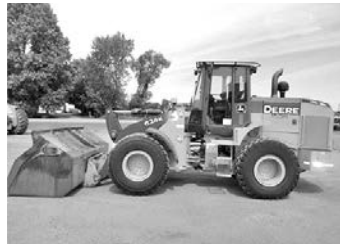
'14 Deere 624K, whl. ldr., 6-yd. tipout (hi-tip/roll-out) bucket, tight center & bucket linkage, 23.5x25 tires 40%, 4 spd. powershift trans. .... $94,500
