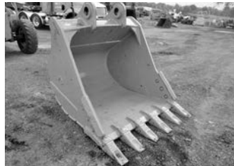
EMAQ 60" Cat 345 GP bucket , for Cat 345 TB linkage, 110mm pin hole & 100mm pin hole w/17-1/4 between ears & 23-1/2 center to center. .... $6,950
