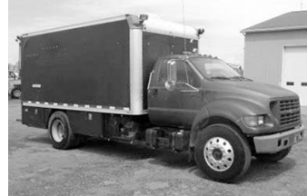
Ford F750XL fuel & lube truck, Cat dsl., Allison auto. trans., 16' Supreme enclosed box, 140-gal. dsl. fuel, (3) 280-gal. tanks, (3) 50-gal. tanks, waste oil tank, hyd. driven product pumps . . $24,500
