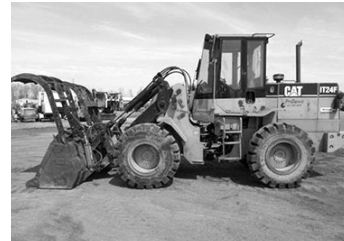
Cat IT24F , cab, heat, A/C, 2.25 yd., G.P. grapple bkt., 175x25 L5 rock tires, quick coupler, aux. & hi-flow hyd., minor rust, call for more details ..... $29,500
