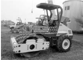
'07 Bomag BW145DH-3, 56" pad foot, drum roller, tires @ 90%, drum drive, vibratory, Duetz dsl., canopy, alarms & lights all work, tight center, like new..... $34,500
