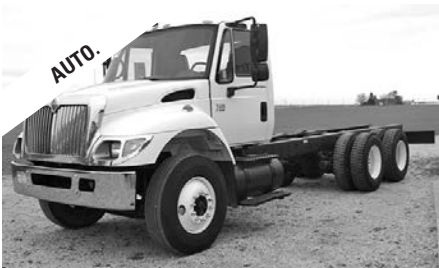
'07 Int'l. 7400 tdm. chassis, Int'l. DT466, 285 hp, Allison auto. w/PTO, 14F, 40R, Hend., dbl. frame, 138,000 miles, stk. #1567.
