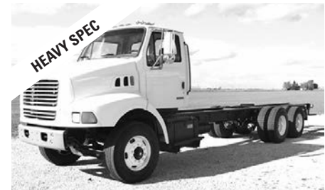
'00 Sterling tdm. chassis, Cat 275 hp, 8LL trans., 18F, 40R, TuffTrac susp., 220,000 miles, 28' of frame, stk. #1609, $19,900.
