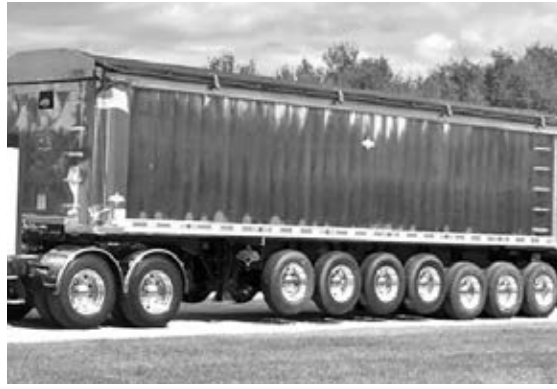
'18 Trailstar 38'x102"x86" 7-axle frt. to back Shurco tarp, liner, push bloc, 11x22.5 tires, (3) down & (4) up. (989) 205-2548
