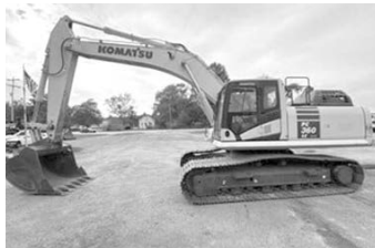
'16 Komatsu PC360 LC-11 , cab, heat, A/C, clean straight orig. machine, long & wide U/C, digital dash, rear camera, long stick, 60" bucket, 3-yd. cap. .... $167,500
